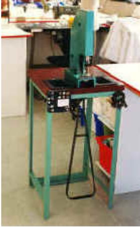
KPR1 is a foot operated ratchet press. It is supplied complete on a stand which incorporates two side trays for stud part storage. It is designed to attach most press fasteners, rivets eyelets, jeans buttons etc. It is extremely versatile and can be used for placing piercing trim on textiles or paper and card. We can supply a full range of dies, which are made in the UK of hardened & tempered steel to fit our own ranges or your existing studs or eyelets.
